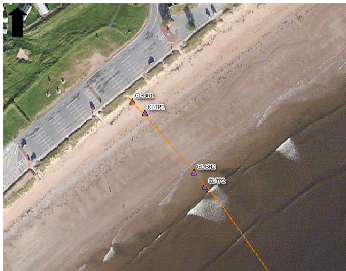
FIGURE 8: Location of site investigation works at Claycastle Beach (possible route of cable is shown in orange)
