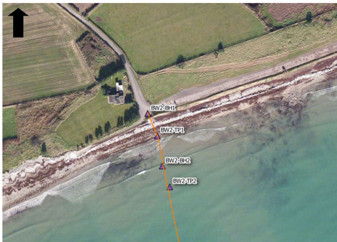
FIGURE 6: Location of site investigation works at Ballinwilling Beach (possible route of cable is shown in orange)
