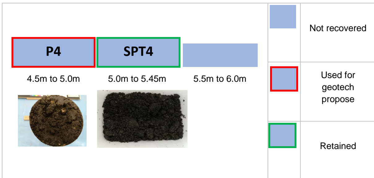
Figure 37 Samples from CL-BH1 (from Next GeoSolutions)
