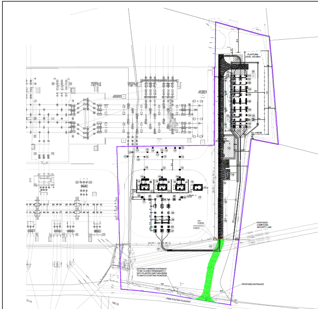
Proposed Site Layout – new internal vehicular access and entrance at the Knockraha CSE compound
